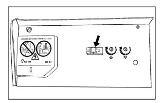
Locate in the garage, the garage door opener receiver (motor-head unit). Locate the "Learn" or "Smart" button. It can usually be found where the hanging antenna wire is attached to the motor-head unit and may be a colored button. Press this button. After you press this button, you will have 30 seconds to complete the following steps.
